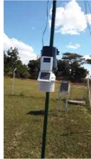
Vantage Station capable of monitoring wind speed and direction, temperature, humidity, wind chill, dew point, rainfall, barometric pressure and forecast FARS solar and UV sensors
