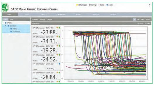
Figure 2.1: Screenshot of the SPGRC Genebank freezer temperature monitoring system.
